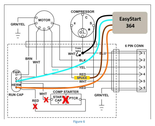
Figure 6 shows the typical wiring diagram supplied with the Brisk I. The red X's indicate components that will be removed during installation of EasyStart. The white wire from EasyStart is drawn in blue for contrast.
