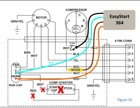
Figure 15 shows a quick synopsis of the changes made to the wiring. The red X's show the compressor start capacitor and PTCR that will be removed during installation. Please note that many if not all Brisk II models do not have a compressor start capacitor or PTCR so this can be ignored in most installations. To be sure, simply check the red wire terminal (HREM terminal) on the run capacitor. If you have only one red wire and no other wires, there is no start circuitry to remove.
