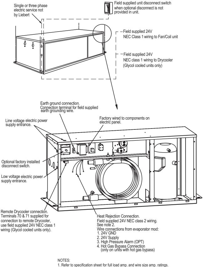
2. Control voltage wiring must be a minimum of 16 GA (1.6mm) for up to 75' (23m) or not to exceed 1 volt drop in control line.
