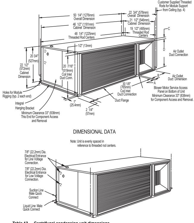
Figure 10 Centrifugal condensing unit dimensions and pipe connections (2 and 3 ton)
