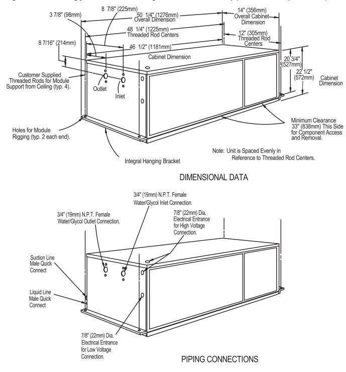
Figure 15 Water and glycol cooled condensing units: dimensions and pipe connections (2 and 3 ton)
