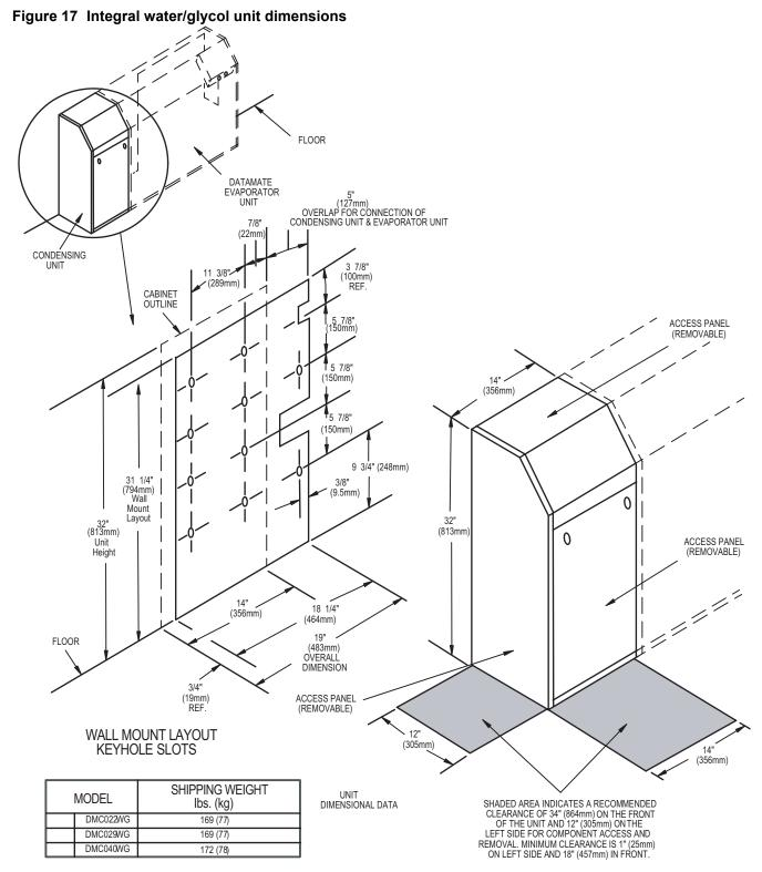
Unlatch the front cabinet door and remove the two screws that secure the cabinet to the chassis. Lift off the cabinet. Eight keyhole slots are provided for mounting the unit on the wall (refer to **Figure 17**).
