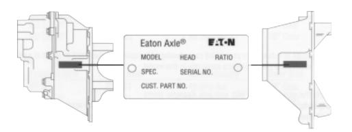
• Axle Housings are identified by the specification number stamped on the rear right-hand side of the axle housing. This number identifies all components of the axle as built by Eaton, including OEM special requirements such as yoke or flange. Some axles may also include an identification tag as shown.
