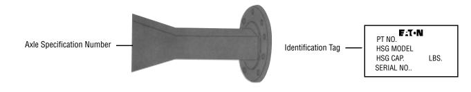
• The axles illustrated in this book are found on a number of different axle shafts, according to OEM specifications. When ordering replacement axle shafts, note the part number stamped into the flange.
