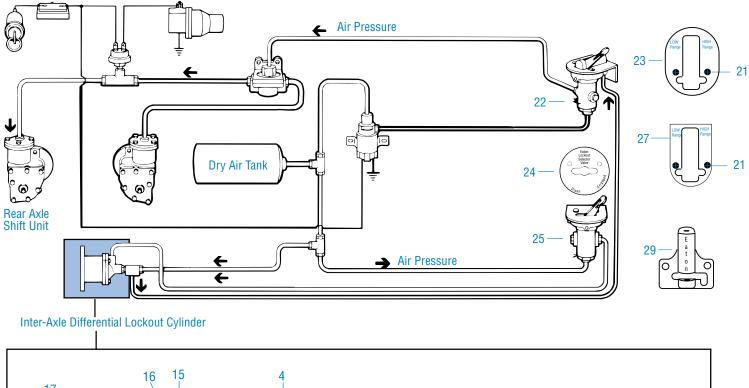
Axle Range Selection and Inter-Axle Differential Lockout System with Axle Range Interlock and Straight-air type Lockout
