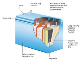
Figure 2. Internal and external components of a valve-regulated lead acid (VRLA)
