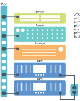
ATSs provide power redundancy to equipment with only one power supply. The ATS automatically transfers the power from a primary source to a secondary source if there is a problem with the primary. Once the primary source is restored, power transfers back through it.
