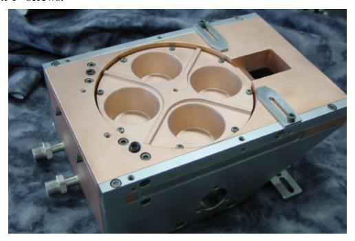
Next, mount the (2) Pole Extensions (EB-2421)with (2) 10-32 x 3/8" screws and install (2) O Rings (2-106) into the Coil Housing (EB2-2404)
