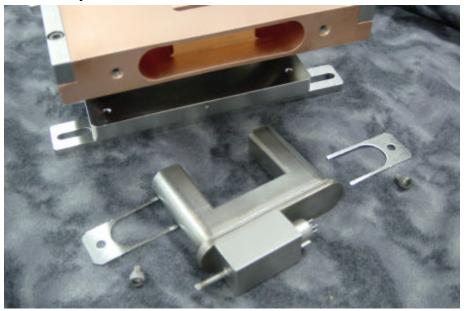
Note: Mount the drive onto your source with (3)  $10-32 \times 3/8$ " screws before installing into your system.
