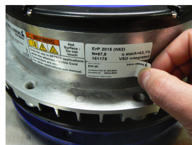
Sticking the EM-W inside label on the ECblue housing.
