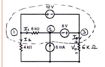
KCL at supernode:  $6m = I_2 + I_0$  $\frac{V_1}{4k} + \frac{V_3}{6k} = 6m$
