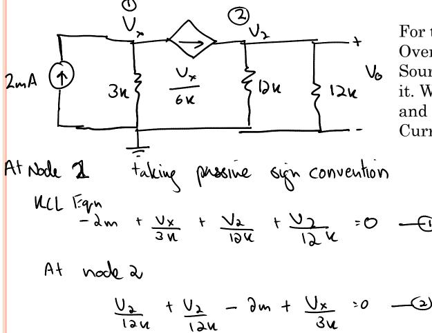
For this Circuit, We need to Overlook the node with dependent Source and form equations round it. We use KCL at Nodes 1 and 2 and derive the equations based on Current flow.
