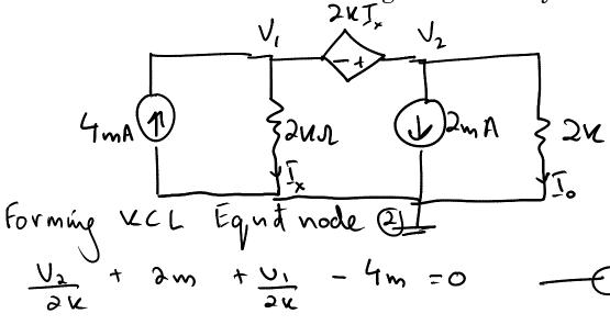
Using KCL at nodes 2 and Forming a controlling equation At node 1 we can simplify the Problem into simple equations. Current entering the node is Summed at the node to form The equations.
