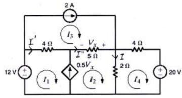
$$\begin{aligned} & \text{KCL} : I_1 = I' + I_3 \\ & I' = I_1 - I_3 \\ & \text{KCL} : I + I_Y = I_2 \\ & I = I_2 - I_Y \\ & \text{KCL} : I'' + I_3 = I + I_Y \\ & I'' = -I_3 + I_Y + I_2 - I_Y \\ & I'' = I_2 - I_3 \end{aligned}$$
