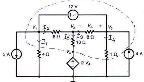
KCL at (2):  $I_2 = I_5 + I_3$  $\frac{V_1 - V_2}{6} = \frac{V_2 - V_4}{10} + \frac{V_2 - V_3}{8}$
