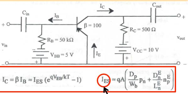
The is independent of the output so long as  $V_{CB} < 0$ . But what is the dc operating point? Sum dc voltages around loop:  $V_{BB} = V_{EB} + I_B R_B$   $U_{BB} = V_{EB} + I_B R_B$   $U_{BB} = V_{EB} + I_B R_B$   $U_{BB} = 0.10$   $V_{BB} = 0.10$  $V_{BB} = 0.10$
