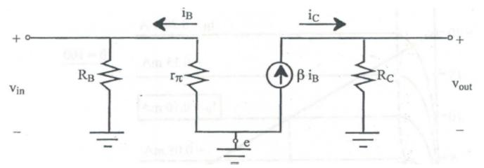
The differential conductance of the forward biased emitter junction is given by the slope of the input characteristic at the dc bias point:
