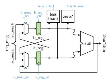
Figure 32: Datapath Diagram for GCD - Datapath in-
