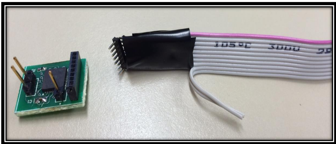
Figure 3.8: PFG Sensor (Left) and Custom 8-pin Plug-and-Play Connector (Right)
