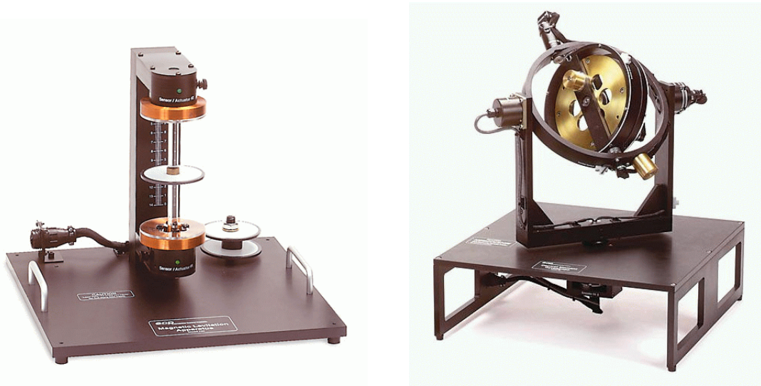
Figure 1.1 The two lab devices. The MagLev device is to the left; the Gyro device is to the right.
