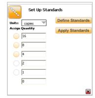
2 Enter the number of points in the standard curve, the quantity of the most concentrated standard, and the desired dilution factor, and then click .
