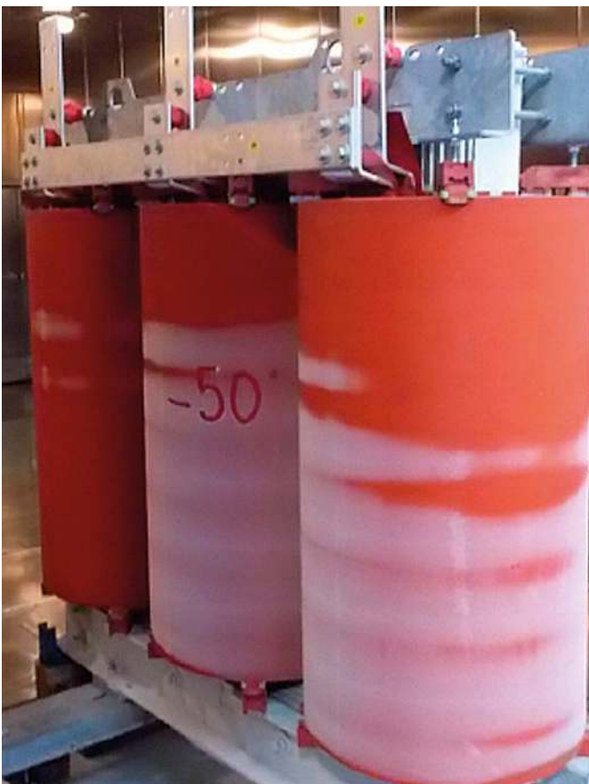
Tesar Transformer during climate test
