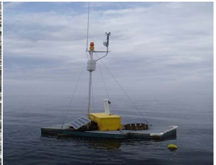
Figure 8. Autonomous vertical profiler deployed in the Neuse River Estuary as a key component for tracking the impact of extreme storm events ( Photo credit: Rachel T. Noble, UNC Chapel Hill ).
