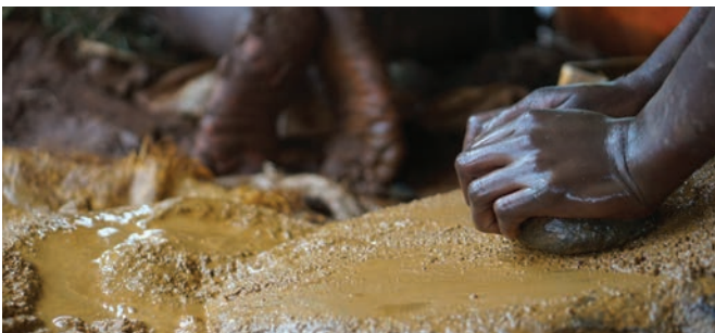
An artisanal miner removes clay deposits using a manual hand-scrubbing method. Processing artisanal gold is very labor-intensive, and sometimes mechanization is not sustainable on small-scale sites.
