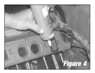
With the Edelbrock intake manifold, you must use RTV High Temp silicone sealer instead of end seal gaskets. Apply a 1/4" thick bead of sealant across each end seal surface (See Figure 5).
