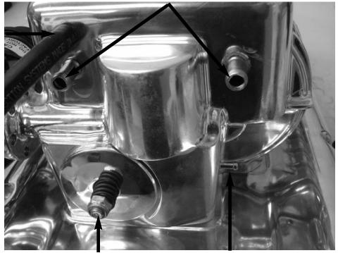
**Sneeze Valve:** Prevents engine damage in the event of an engine backfire. Leave as loose as possible without experiencing a dropoff in boost pressure.
