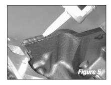
Carefully install the intake manifold onto the engine, making sure the ports and bolt holes line up with the gasket. For 1986 and earlier applications, you may install the intake manifold bolts.
