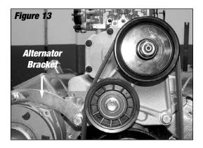
B. Install the idler pulley onto the bracket. Use the remaining 3/8-16 x 4" long x 2.75" shoulder bolt, idler pulley spacer, and square idler pulley nut to attach the idler pulley to the bracket (See Figure 14). Make sure the nut is aligned with the slot on the back of the bracket.
