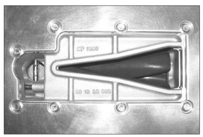
SUPERCHARGER TO TOP PLATE BOLTS. DO NOT REMOVE!
