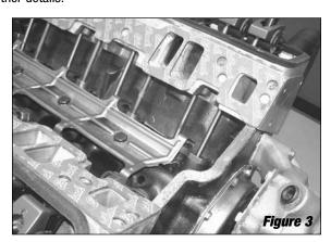
With the intake gaskets in place, apply a small amount of RTV High Temp silicone sealer around the water passages on the intake manifold side (See Figure 4).
