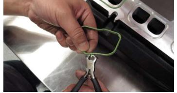
52. Apply silicone lubricant to the modified O-ring gaskets then insert the gaskets into the supercharger runner as shown.
