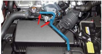
14. Disconnect the MAF sensor harness from the MAF sensor. Using a panel puller, remove the plastic retaining pin from the airbox lid.
