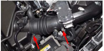
133. Reconnect the coolant bleed hose to the radiator fill neck and lock the hose into place with the retaining clip on the airbox.
