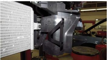
94. Using an appropriate cutting tool, remove the top corner of the passenger side radiator shroud to allow for water pump hose clearance. Use the red line and measurements below for reference.
