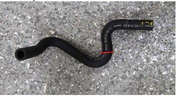
119. Attach the two (2) factory EVAP hose clamps onto the hose cut in the previous step in the locations shown below.
