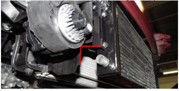
103. Using three (3) 3/4" clamps and one (1) straight connector from Bag #2, install the hose (highlighted blue) from the bottom fitting on the LTR to the hose end labeled "Z". Attach convoluted tubing (highlighted red) on the hose where it makes contact with metal or sharp surfaces and secure with zip ties or electrical tape. **NOTE:** *Zip Tie the hose to the two (2) ears on each side of the steering rack to hold it in place.*
