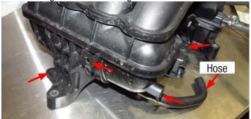
43. Remove the intake manifold and set aside. Using a lint free shop rag, clean the area around the intake ports and cover the ports with masking tape to keep out any debris.
