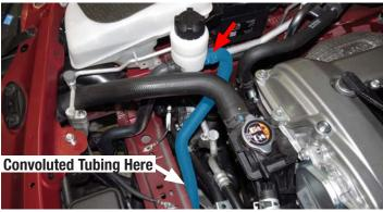
107. Using two (2) 3/4" clamps and one (1) straight connector from Bag #2, attach the hose end labeled "Y" to the end labeled "X" as shown below.
