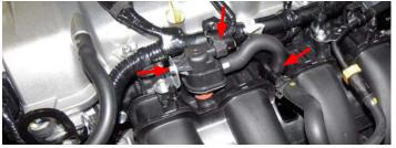
31. Using an 8mm socket, remove the bolt securing the fuel line bracket to the intake manifold.
