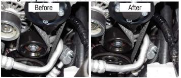
88. Install the surge tank onto the surge tank bracket using the two (2) M6 x 10mm bolts located in Bag #2.
