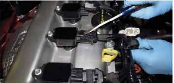
33. Disconnect the fuel pump harness connector at the back of the engine just under the cowl.
