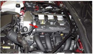
12. Disconnect the valve cover breather hose from the valve cover.
