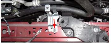
50. Using a 17mm wrench, slowly release the tension on the main drive belt and remove the belt. The wrench should be rotated counter clockwise to compress the tensioner.
