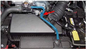
134. Reconnect the MAF sensor harness to the factory MAF sensor on the airbox lid. Also reinstall the harness retaining pin into the hole on the airbox.
