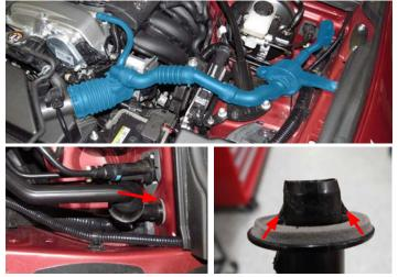
19. If the sound tube was removed, install the included fire wall plug located in hardware Bag #3.
