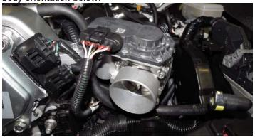
117. Locate the 2' section of hose previously attached to the supercharger inlet during step 72. Push the hose onto the nipple at the bottom of the factory EVAP solenoid.
