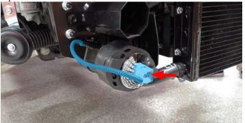
111. Route the power wire and EVAP/engine wires behind the engine coolant reservoir and over to where the battery is normally located. Attach the harness to existing harnesses and secure with zip ties or electrical tape.
