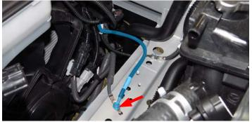
110. Route the connector labeled "water pump" down to the water pump and plug the connector into the pump. Make sure the connector "clicks" into place. Attach the harness to existing harnesses and secure with zip ties or electrical tape.
