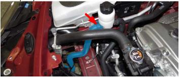
105. Using one (1) 3/4" Hose clamp form Bag #2, secure the surge tank to water pump hose (highlighted blue) to the water pump. Attach convoluted tubing (highlighted red) on the hose where it makes contact with metal or sharp surfaces and secure with zip ties or electrical tape.
