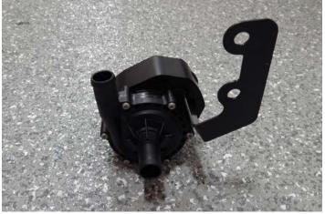
100. Install the water pump and bracket assembly onto the factory studs protruding from the passenger side crash beam support. Using a 13mm socket, secure the bracket to the studs with the two (2) M8 x 1.25 nuts from Bag #2.
