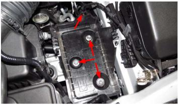
125. Using a 12mm socket, reinstall the two (2) bolts securing the airbox mounting tray.
