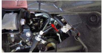
26. Separate the EVAP line and Fuel line by prying apart the plastic clip holding the lines together.
