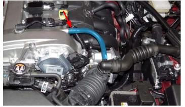
13. Remove the coolant bleed line from the retaining clip and disconnect the hose from the fill cap side.
