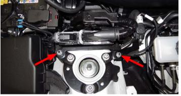
122. Install the EVAP mounting bracket onto the ECM mounting stud closest to the firewall and loosely secure with the factory nut. Attach the EVAP solenoid to the bracket using the factory bolt removed during step 30. Tighten both the nut and bolt.
