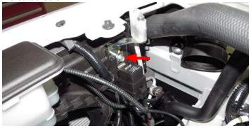
109. Remove the factory ground bolt located on the cross member. Using the factory bolt, secure the wire labeled "ground" on the water pump harness to the factory ground location indicated below.
