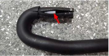
137. Locate the 3' section of hose attached to the supercharger inlet during step 72. Lubricate the brake booster check valve with silicone lube and **insert the tapered end into the hose first**. Push the remaining potion of the check valve into the hose so it sits just below the hose end.
