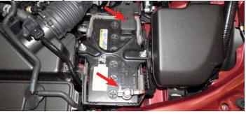
2. Using a 10mm deep socket, remove the battery hold down and set aside. Remove the battery and insulation from the engine bay.
