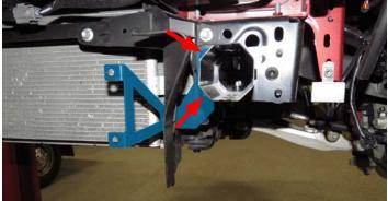
93. Reinstall the driver side shroud using the factory hardware.
