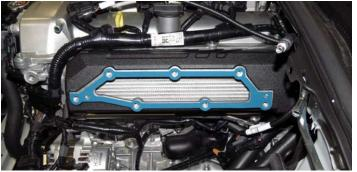
74. With the help from an assistant, lower the supercharger assembly into the engine bay angling the back of the supercharger in first. At this time, attach the previously installed crank case breather hose to the fitting on the back of the supercharger assembly using one (1) 3/8" hose clamp from Bag #2.
