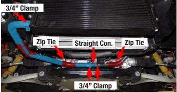
104. Using one (1) 3/4" clamp from Bag #2, secure the surge tank to water pump hose to the surge tank (end labeled "ST") and route the end labeled "WP" down to the water pump.
