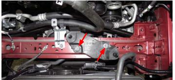
49. Using a 10mm socket, remove the bolt securing the cooling hose bracket to the frame. The bracket can be left attached to the hose. This will make removal/installation of the belt easier.
