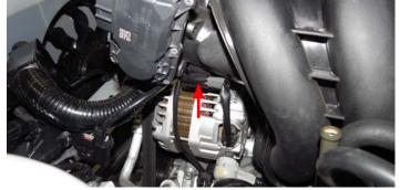
40. Lift up the front of the intake manifold and remove the anchor securing the engine harness to the intake manifold. **NOTE:** *This pin will be located just behind the alternator.*
