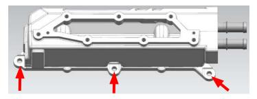
63. Using the torque sequence below, tighten all five (5) supercharger runner bolts to approximately 16 lb-ft.
