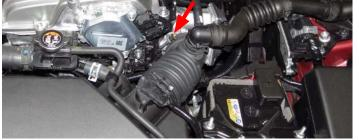
17. If equipped, use a 10mm socket to remove the two (2) bolts securing the sound tube.
