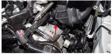
41. Position the intake manifold as far forward as possible and remove the MAP sensor harness connector at the back of the manifold. Using a panel puller, remove the harness anchor attached to the intake manifold next to the MAP sensor.
