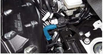
121. Reinstall the ECM and mounting bracket onto the studs protruding from the strut mount.
