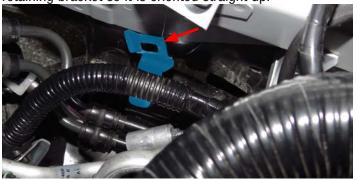
©2017 Edelbrock LLC Part #1554, 15540 57. Position the hose labeled "IC" into the engine bay so that the hose routes under the clutch line (if equipped), engine harness, A/C line and front sway bar.
