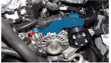
82. Using a 12mm socket, remove the front bolt securing the A/C compressor to the engine. **NOTE:** Pulley removed for photo. *DO NOT remove supercharger pulley.*
