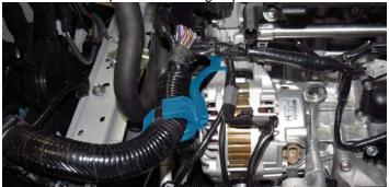
72. Using two (2) 3/4" hose clamps from Bag #2, connect the 2' section of 3/8" hose to the front fitting on the supercharger assembly. This hose will connect to the EVAP solenoid later. Connect the 3' section of hose to the rear fitting. This hose will connect to the brake booster later.
