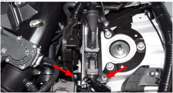
124. Using a 12mm socket and long extension, reinstall the three (3) bolts securing the battery tray to the frame. Also reconnect the retaining pin locating the negative battery terminal to the tray. Make sure the tray clears the modified A/C line.
