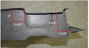
150. Using the factory hardware, reinstall the modified under tray by first rotating the notched section up and around the intercooler hose. One bolt will not be used as the hole was cut away during step #149. **TIP:** *Use a 10mm ratcheting wrench to tighten the bolt above the hose.*
