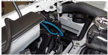
112. Route the MAP sensor harness (installed during step 68) around the driver side of the supercharger and connect the harness to the MAP sensor located on the front of the intake runner.
