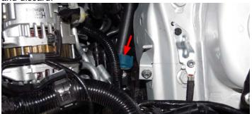
56. Using pliers, bend the top portion of the harness retaining bracket so it is oriented straight up.
