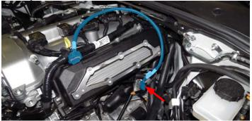
69. Using the one (1) M8 x 20mm bolt from bag #3, loosely install the supercharger support bracket onto the engine block above the drive side engine mount. **NOTE:** *The bracket should be rotated toward the alternator so to rests against the engine mount.*
