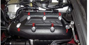
80. Attach protective convoluted tubing (highlighted red) to the engine harness above the alternator so no wires are visible. Secure the convoluted tubing with zip ties or electrical tape.
