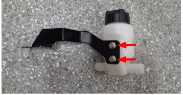
89. Using a 10mm socket, remove the two (2) nuts securing the factory harness connection to the passenger side strut tower. Secure the surge tank bracket to the harness mount using factory nuts.
