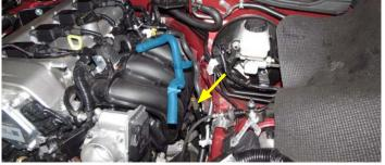
28. Stuff shop rags under the fuel line to catch any spilt fuel and disconnect the line by pulling up on the yellow locking tab.
