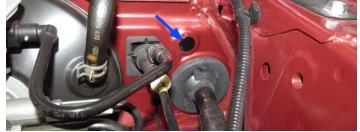
20. Using a 10mm socket, remove the bolt securing the lower portion of the airbox to the frame and remove the airbox. The air inlet tube on the left will remain in place.
