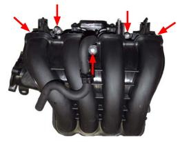
39. Using a panel puller, remove the anchor securing the alternator harness to the intake manifold.
