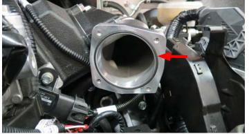
116. Using the factory bolts, install the throttle body onto the supercharger inlet and plug the throttle body extension harness into the throttle body connector. Note the throttle body orientation below.
