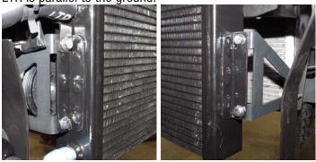
97. Tighten the passenger side radiator shroud bolt left loose in step 95. **TIP:** *This bolt can be reached from the back side of the LTR using a 10mm wrench.*
