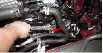
51. Remove the four (4) intake O-ring gaskets from the factory manifold and trim off the small tab on each gasket.
