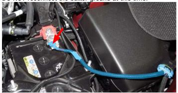
142. Using zip ties, secure all water pump harness wires away from any moving parts or potentially hot surfaces. Secure the water pump fuse holder inside the fuse box next to the battery as shown below and reinstall the lid.
