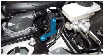
123. Secure the ECM mounting bracket to the vehicle with the remaining nut and bolt removed during step 23. Reattach the black box to the side of the ECM bracket and reconnect the two (2) engine harness connections to the ECM.
