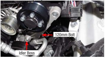
84. Secure the idler bracket to the supercharger nose using the 25mm socket head bolt from Bag #1. Tighten both idler bracket bolts to 18 lb/ft.
