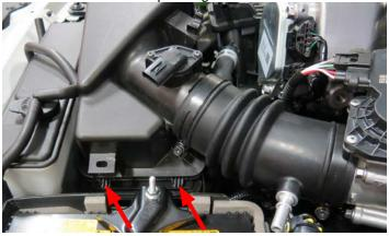
131. Connect the valve cover breather hose to the fitting on the intake tube by pushing the connector onto the fitting until it "clicks" into place.
