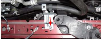
127. Using the factory hardware, reinstall the lower portion of the airbox and insert the provided K&N high flow filter in place of the factory paper filter.
