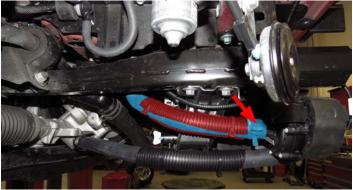
106. Using one (1) 3/4" clamp from Bag #2, install the hose (highlighted blue) to the surge tank (end labeled "ST"), and route the other end of the hose (labeled "Y") down toward the steering rack. Attach convoluted tubing where the hose touches the frame.
