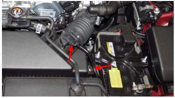
15. Disengage the two (2) clips retaining the airbox lid and loosen the clamp securing the rubber intake tube to the lid. Remove the lid and air filter and set aside.
