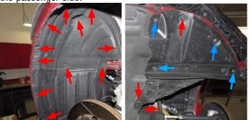
7. Using A 10mm socket, panel puller and Phillips Head Screwdriver, remove the eight (8) bolts, two (2) screws and two (2) push pins securing the under tray.
