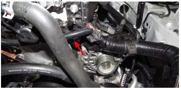
71. Using a flat head screwdriver, separate the plastic retaining clip from the engine harness. Remove and discard the bracket and plastic retaining clip.
