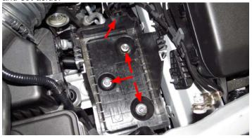
4. Using a panel puller and Phillips head screwdriver, remove the four (4) push pins and two (2) screws securing the radiator cover to the frame.
