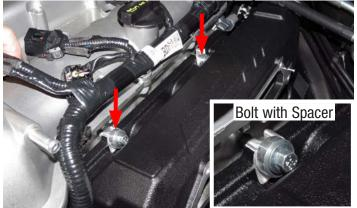
62. Insert the three (3) M8 x 25mm Hex Flange bolts from Bag #3 into the lower holes on the supercharger runner. Use a small 10mm swivel to snug all three bolts.
