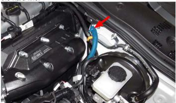
139. Route the EVAP connector on the water pump harness to the EVAP solenoid and connect as shown. Attach the harness to existing harnesses and secure with zip ties or electrical tape.
