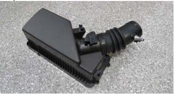
130. Reinstall the airbox lid making sure the tabs on the lid engage into the slots on the lower portion of the airbox. Once in place, lock the two (2) clips securing the lid to the lower half of the box. **NOTE:** *The intake tube should be installed onto the throttle body at the same time the lid tabs are slid into their corresponding slots.*
