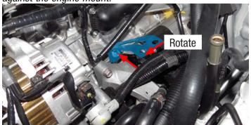
70. Using a 14mm socket, remove the top bolt securing the alternator to the engine block.
