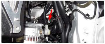
65. Using the factory bolt removed during step #24, loosely secure the transmission cooling hose bracket to the frame. Attach the provided hose clamp around both hoses and secure the clamp to the bracket with the factory bolt removed during step #64. Tighten both bolts.
