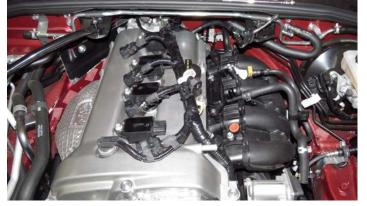
38. Using a 10mm socket and long extension, remove the five (5) remaining intake manifold bolts securing the manifold to the cylinder head. **NOTE:** *Do not remove the intake manifold as the engine harness is still attached.*
