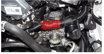
81. Install the provided engine harness retention bracket using the factory alternator bolt. Torque bolt to 32 lb/ft.
