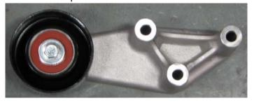
53. Use a 10mm socket to remove the three bolts on the passenger side of the water pump.
