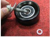
72. Apply Loctite to the threads on both idler pulley bolts. Then use a 15mm socket to install the 76mm idler pulley with the factory hardware to the left idler pulley location. Install the additional idler pulley to the right idler pulley location with the M8 x 20mm bolt and M8 washer from Bag #1. Torque both pulley bolts to 18 ft-lbs. Verify that both pulleys spin freely.
