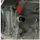
31. Apply thread sealant w/ PTFE to the threads on the plug removed from the engine block and install it to the factory oil sensor location.
