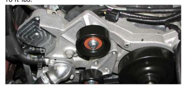
67. Apply blue Loctite to the threads of the M10 x 75mm Hex flange bolt supplied in Bag #1. Use a 15mm socket to install the supplied tensioner onto the tensioner bracket. Torque bolt to 37 ft-lbs.
