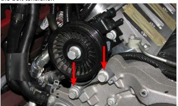
61. Apply blue loctite to the threads of one M8 x 20mm bolt supplied in Bag #1, then use a 12mm socket and a supplied M8 washer, from bag #1, to mount the pulley onto the new lower idler bracket. Torque bolt to 18 ft-lbs.
