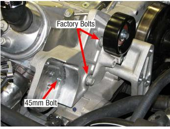
56. Apply blue loctite to the threads of one M8 X 20mm bolt supplied in Bag #1, then use a 12mm socket and the supplied washer to mount the pulley on the tensioner bracket and torque it to 18 ft-lbs.
