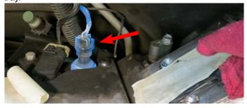
30. Using a 8mm Allen wrench, remove the factory plug towards the front driver side of the block, adjacent to the crank pulley. Apply thread sealant w/ PTFE to the threads of the factory oil pressure sensor and install the sensor in the location of the plug. Torque to 26 ft/lbs (35 Nm).
