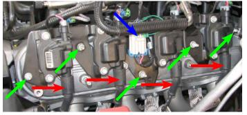
6. Engines using the Corvette front accessory drive setup will need to remove the power steering reservoir and determine an alternate mounting location due to interference with the supercharger snout. Inspect the engine bay for any other items that may interfere with the installation of the supercharger.
