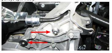
73. Route the serpentine belt (*not included*) using the diagram below. Use a 15mm socket to release tension from the tensioner and re-tension after the belt is routed. Proceed to Step 74.
