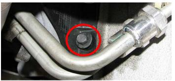
9. Use a 13mm socket to remove the two starter bolts.
