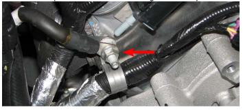
65. Install the supplied tensioner bracket to the water pump using the spacers from bag #6, three M10 x 65mm bolts from bag #1, and blue Loctite. The two short spaces go onto the two provisions on the water pump with two 65mm hex flange bolts, and the long spacer goes on the cylinder head provision with the 65mm socket head bolt.
