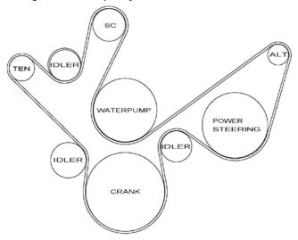
59. Use a breaker bar and a 16mm socket to release the tension on the tensioner enough to get the belt on. Double check the routing and make sure the belt is seated properly. Proceed to Step 74.
