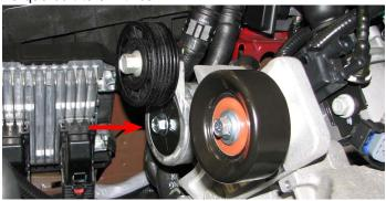
68. Use a 12mm socket and an M8 x 20mm bolt supplied in Bag #1 to secure the ground strap to the back side of the tensioner bracket.
