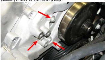
54. Using a 6mm Allen tool and the three M8 x 90mm bolts supplied in Bag #1, install the lower idler bracket onto the water pump then torque them to 18 ft-lbs.
