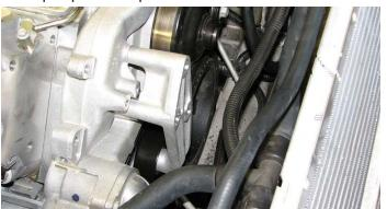
55. Apply blue Loctite to two stock tensioner bolts which were removed during Step 53. Mount the new tensioner bracket onto the water pump using the stock bolts and a 15mm socket. Apply blue Loctite to the M10 x 45mm bolt supplied in Bag #1 and install the bolt to the left provision on the bracket. Torque all three bolts to 37 ft-lbs.
