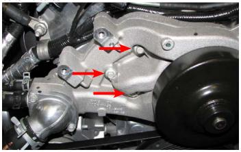
63. Apply blue Loctite to the threads of the M8 x 100mm bolts supplied in Bag #1 then use a 6mm Allen tool to install the idler bracket onto the water pump. Torque bolts to 18 ft-lbs
