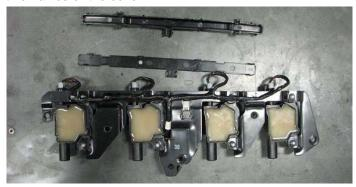
48. Tuck any loose wiring under each coil bracket then use a 10mm socket and the ten stock bolts to install the coil brackets on to each valve cover.
