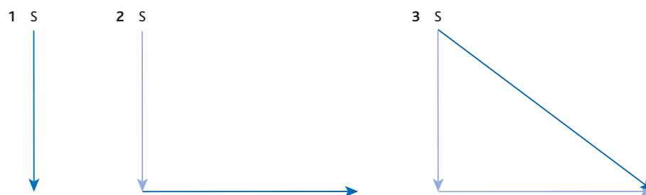
fig. 1.1.12 Adding displacement vectors using a scale diagram. 1 cm represents 10 m.
