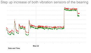
GT cooling blade degradation
