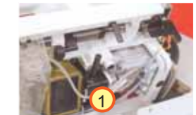
Integrated sewing drive in the Top.
