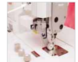
Simple changeover on different puller sizes
