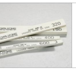
**AM-K** - White Aluminum Oxide Stone Good for Machined Surfaces AM-K is a white aluminum oxide stone of medium hardness that performs well on all types of mold steel. Generally, AM-K is used dry for rough forming and removal of machine marks. Lubricants are used for finer grits. Some polishers use the 400 and 600 grits for finishing plastic molds and blow molds.
