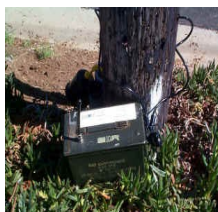
Here's a specially-designed "fox" transmitter used at a hidden transmitter hunt during a Handiham Camp in Ventura County, CA one year. Note the cable that locks it to the tree trunk.
