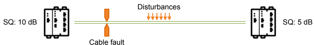
Figure 16: Asymmetric values for signal quality due to one-sided cable fault
