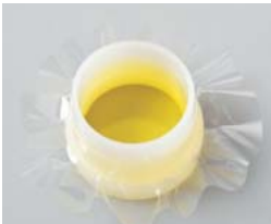
Cover the bottom of the cell with film and add the sample.
