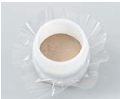
Cover the bottom of the cell with film and add the sample (loose powder method).
