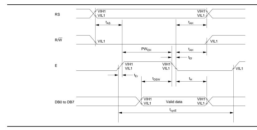
Figure 27 Write Operation
