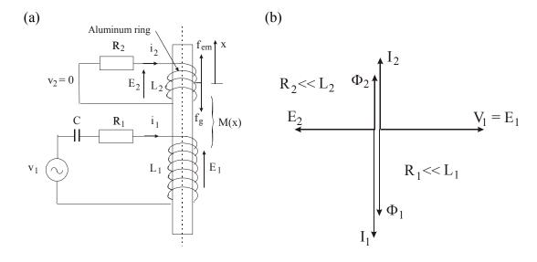
Fig.30 Equivalent circuit of the *jumping ring* (a), and its phasor diagram (b)
