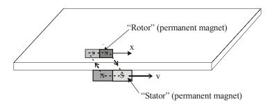
Fig.2 Linear permanent magnet synchronous motor formed by the moving "stator" permanent magnet that is pulling the "rotor" permanent magnet
