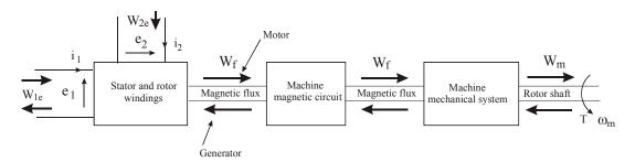
Fig.9 Diagram of electromechanical energy conversion; no power losses are included
