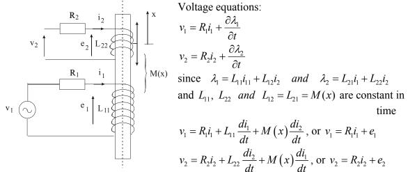
Fig.28 Equivalent circuit of transformer
