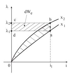
Fig.21 Illustration to the magnetic force derivation
