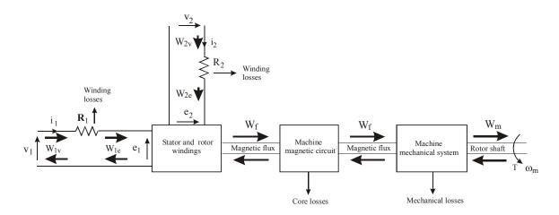
Fig.11 Diagram of electromechanical energy conversion with inclusion of power losses
