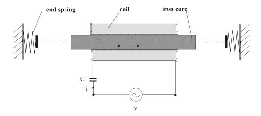
Fig.34 Reluctance linear oscillator with end springs
