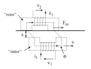
Fig.8 Illustration to electromechanical energy conversion
