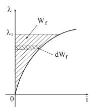
Fig.14 Field energy on  $\lambda$ -*i* characteristic
