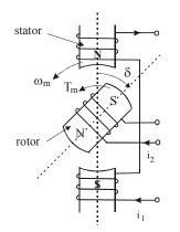
Fig.5 Rotary synchronous motor
