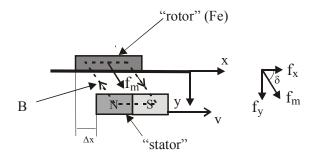
Fig.22 Force components in linear reluctance motor
