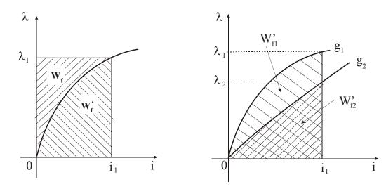
Fig.18 Field energy  $W_f$  and field co-energy  $W_f$ '
