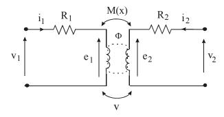
Fig.26 Equivalent circuit of the electromechanical system in Fig.20
