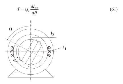
Fig.38 Motor with cylindrical stator and rotor
