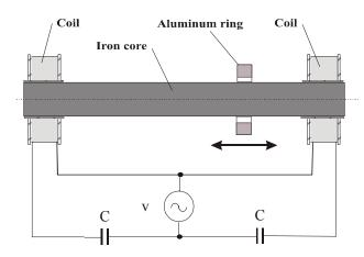
Fig.31 Scheme of induction linear oscillator
