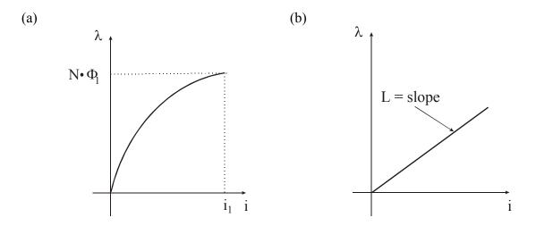
Fig.13 Magnetic linkage-current characteristic for: (a) – nonlinear system, (b) – for linear system
