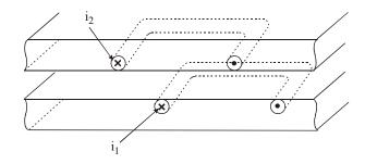
Fig.25 Coils in the infinitely long "stator" and "rotor" cores
