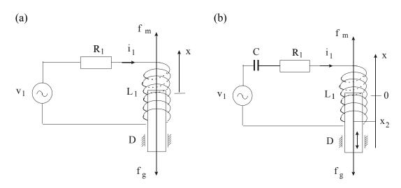
Fig.32 Circuit diagrams: (a) ferromagnetic bar suspended by the magnetic field, (b) electromagnetic device with jumping ferromagnetic bar
