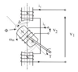
Fig.10 Illustration to electromechanical energy conversion in rotary synchronous generator
