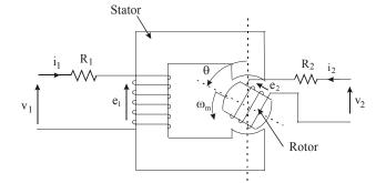
Fig.35 Rotary motor with salient pole stator and rotor
