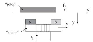
Fig.23 Force component  $F_x$  produced in the linear reluctance motor
