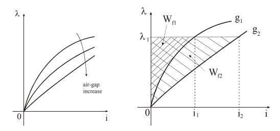
Fig.15 λ-I characteristics for various air- Fig.16 Field energy in the machine with different air-gap
