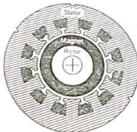
Fig 4.1 Arrangement of permanent magnet in the rotor
