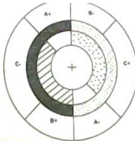
Fig.4.24 BLDC motor with 120° magnet arcs and 180° square wave phase currents
