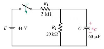
a. Transform the circuit into the Thevenin equivalent circuit as seen by the capacitor.
