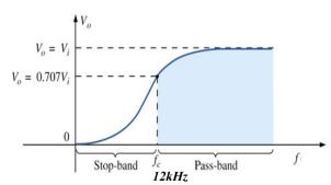
The *stop band* in all filters are the frequencies which are rejected and the *pass band* represents the frequencies which are passed through the system. It is important to be able to identify these on a given filter frequency response. We can build a high pas filter using only two components as shown.
