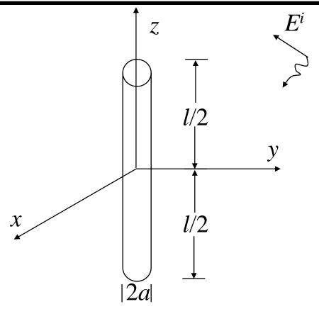
• The target is to determine the current distribution and consequently the scattered field due to an incident field for a finite-diameter wire
