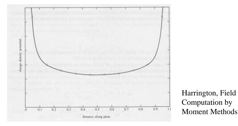
The charge distribution along the width of the plate
