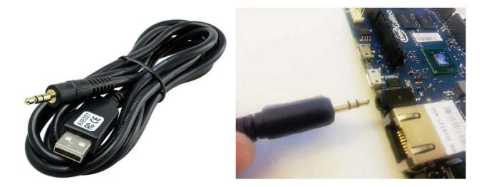
The next step tests the cable with Galileo Gen 1 board. By the way, to run a Linux console with the cable, we need to install the software on a computer in order to pen a serial channel with Galileo Gen 1. The software we need depends on our operational system and our preference. This step explores **putty** for Windows, **minimcom** for Linux, and **screen** for Max OS. Note that **screen** is also available on Linux, and **minicom** is also available in Mac OS.
