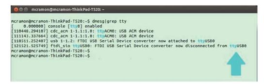
Figure 1-23. Checking the USB port enumerated on the Ubuntu terminal
