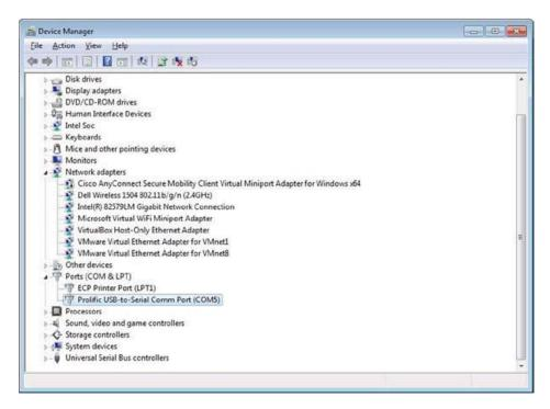
Figure 1-20. Intel Galileo COM port on Windows
