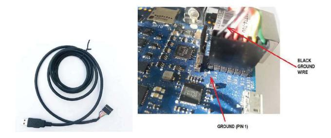
The next step tests the cable with Galileo Gen 2 board. By the way, to run a Linux console with the cable, we need to install the software on a computer in order to pen a serial channel with Galileo Gen 2. The software we need depends on our operational system and our preference. This step explores **putty** for Windows, **minimcom** for Linux, and **screen** for Max OS. Note that **screen** is also available on Linux, and **minicom** is also available in Mac OS.
