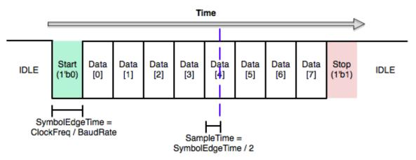
Figure 1: UART Frame Structure
