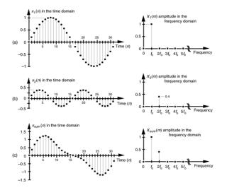
Fourier analysis decomposes signals into sinusoidal components
