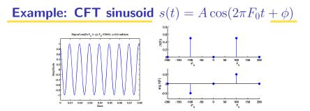
Sinusoid at  $F_0 = 100$ Hz Fourier transform ( $T_0 = 1/F_0$ =period)
