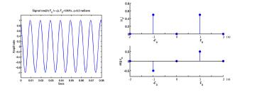
Sinusoid at  $F_0 = 100$ Hz
