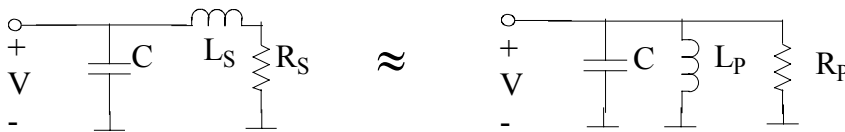
Figure 4.7 Tuned circuit with lossy inductor
