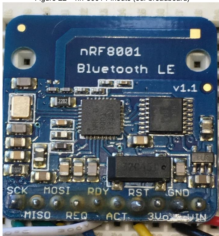
Figure 22 – nRF8001 Pinouts (our breadboard)
