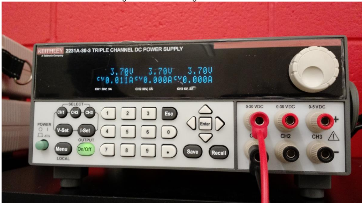
Figure 30 - Measuring Current Draw
