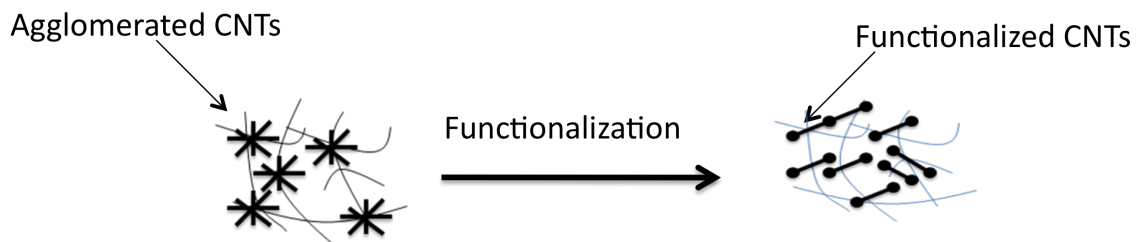
Figure 2.5: Effect of functionalization on the dispersion quality
