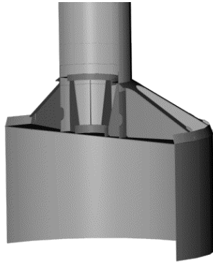
Figure 1. Sectional view of bucket foundation
