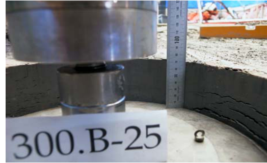
Figure 8. Bucket experiments with 30 cm foundation with 25 % embedment ratio
