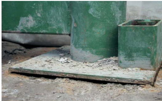
Figure 7. Plate load test on 40 cm circular surface foundations
