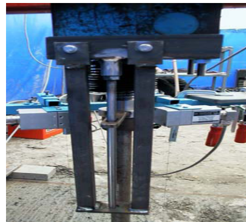
Figure 6. Setting up the hanger bar
