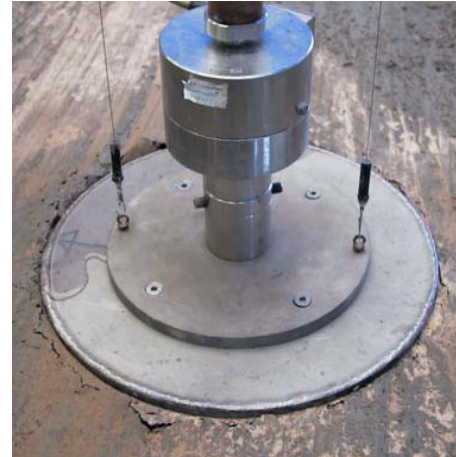
Figure 5. Bucket foundation before and after installation
