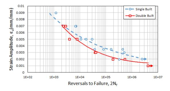
Figure 6. Comparison strain-life fatigue behavior for single and double built LENS Ti-6Al-4V.
