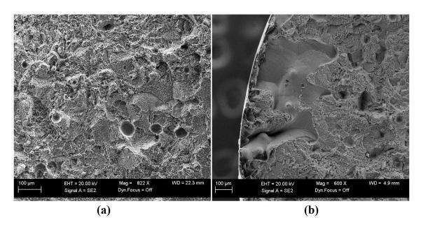
Figure 5. Pores from tensile fracture surfaces of (a) a single built LENS, and (b) a double built LENS Ti-6Al-4V specimen.
