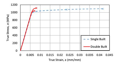
Figure 4. Tensile stress-strain curves for single and double built LENS Ti-6Al-4V.
