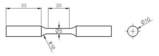
Figure 1. Dimensions of cylindrical tensile fatigue specimens based on ASTM E606 (units in millimeters).
