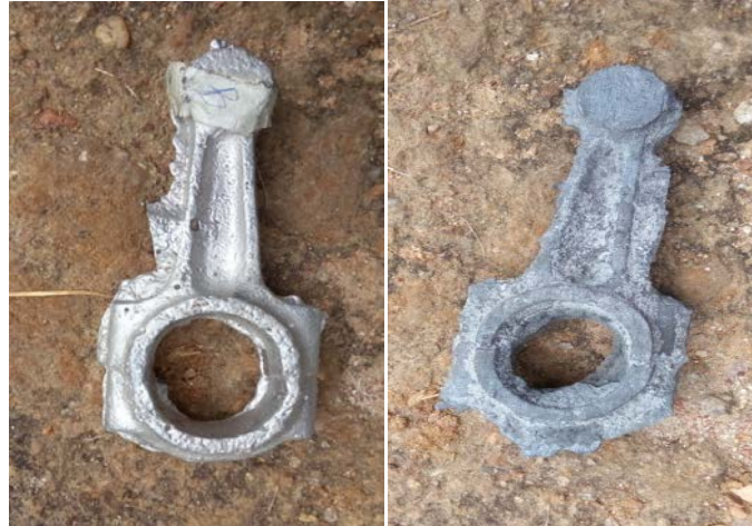
Figure 9: Unmachined motor car connecting rod
