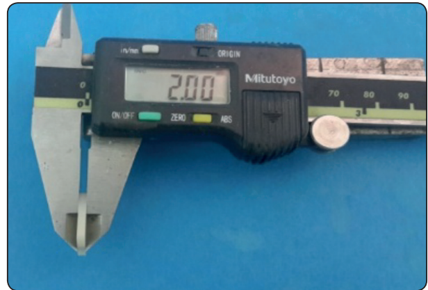
Fig. (2): Empress CAD plates, 2mm thickness
