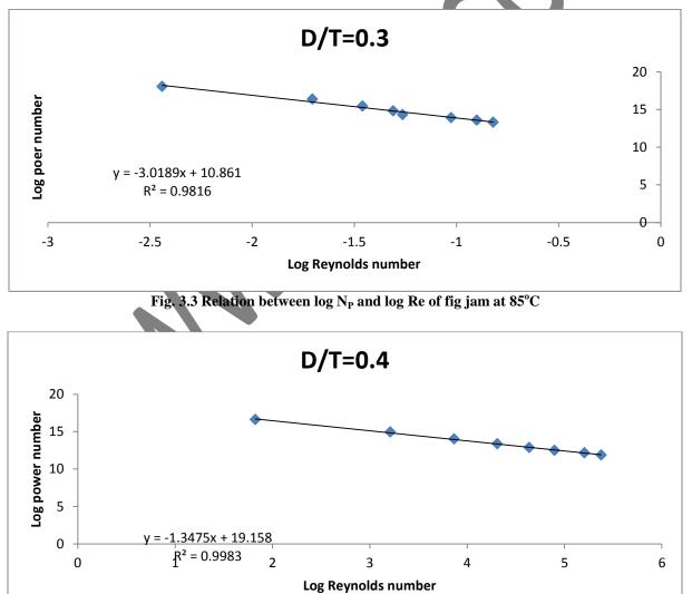
Fig. 3.4 Relation between log  $N_P$  and log Re of fig jam at  $85^{\circ}\mathrm{C}$
