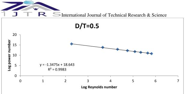
Fig. 3.5 Relation between log N<sub>P</sub> and log Re of fig jam at 85°C
