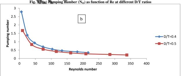
Fig. 3.7 (b) Pumping number (N<sub>0</sub>) as function of Re at different D/T ratios
