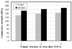
Figure 2. Compressive Strength for Cube Specimens at Age 7 and 28 Days with Different Steel Fibers Volume Fractions and Aspect Ratio Equals 50
