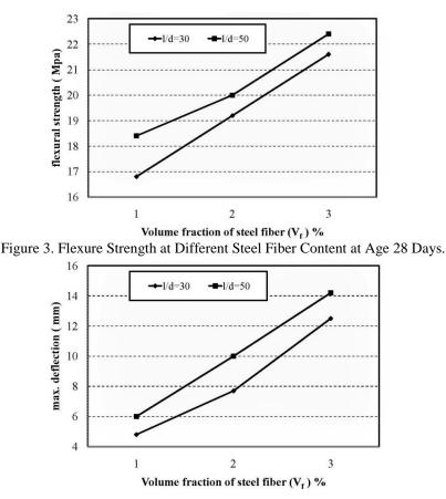
Figure 4.Effect of Steel Fiber on Maximum Deflection.
