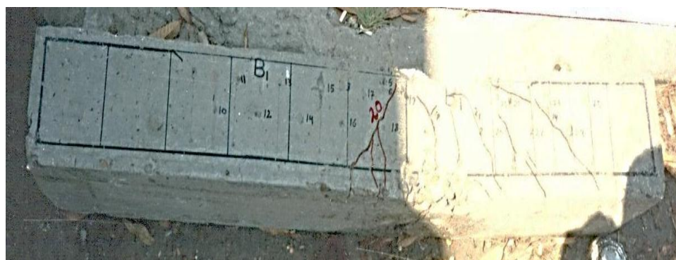
Figure 3 b: Shear Cracks on beam (B 1 ); Flexure Failure
