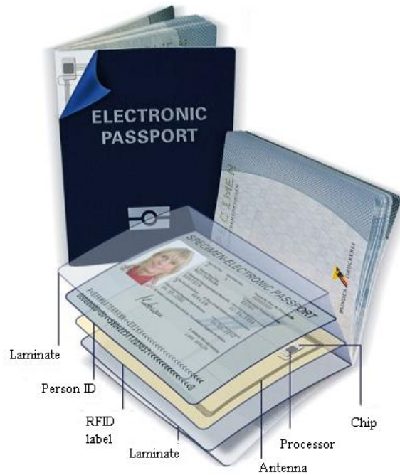
Figure 72 - e-passport architecture courtesy of Bundes Druckerei
