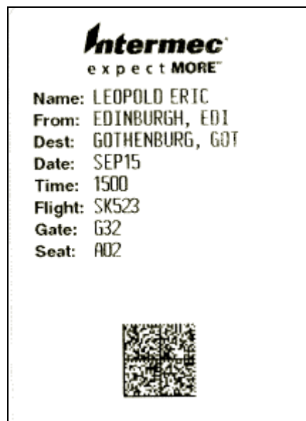
Figure 92 - Sample of BCBP printed on a credit card size stock – Datamatrix code
