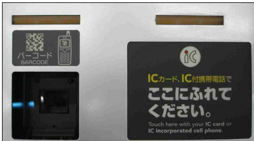
Figure 68 - Kiosk embedded 2D bar code scanner and IC card reader courtesy of JAL
