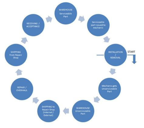
Figure 5. Ideal Component Repair Cycle; Airline TAT
