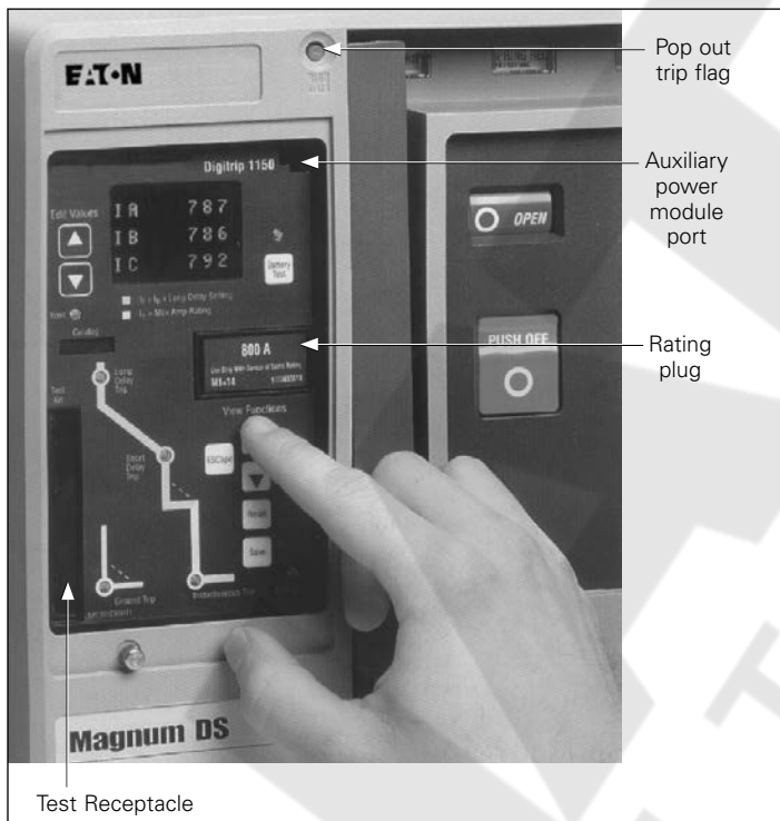
Figure 37. Digitrip RMS 1150 programmable trip unit installed in Magnum DS circuit breaker
