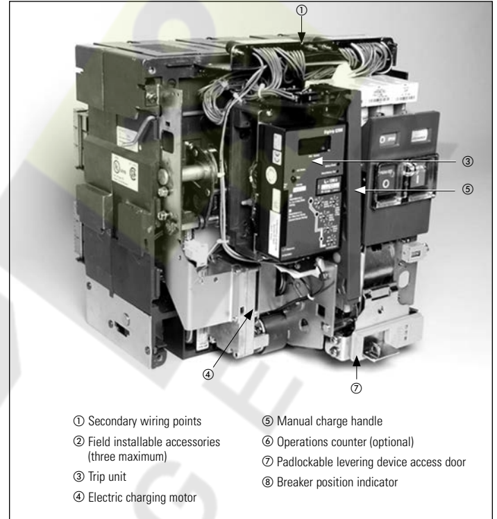
Figure 29. Typical electrically operated drawout MDS/MDSX circuit breaker with front cover removed
