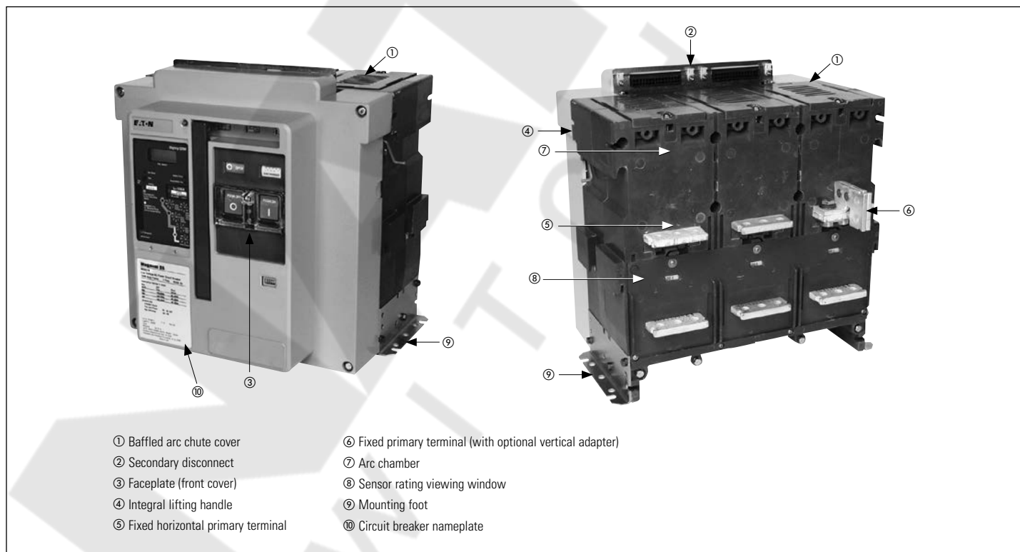
Figure 19. Typical MDS/MDSX fixed circuit breaker features (front and rear views) (MDSX shown without required arc hood)
