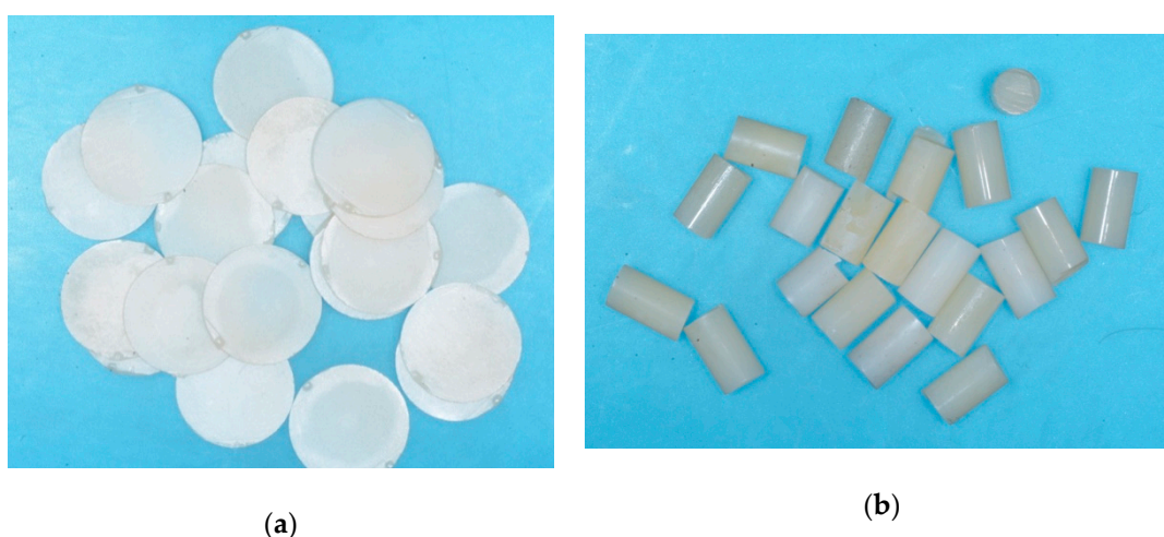
Figure 1. (a) Y-TZP disks used for the study (10 mm diameter, 0.5 mm thick) (n = 20); (b) Nano-hybrid composite cylinders created for the study (4 mm diameter, 8 mm height) (n = 20).
