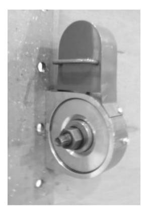
Figure E.1: Rear View of Typical Skidmore Setup
