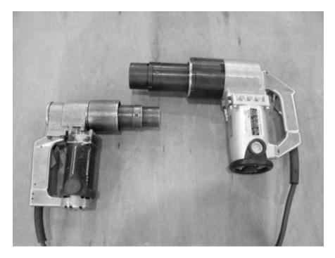
**Figure E.3: Tone Wrenches Used for Tightening**
