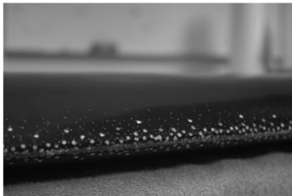
Figure 4. Photograph of the DU 96-W-180 wind tunnel model with Type C/Stage 3 leading edge erosion.
